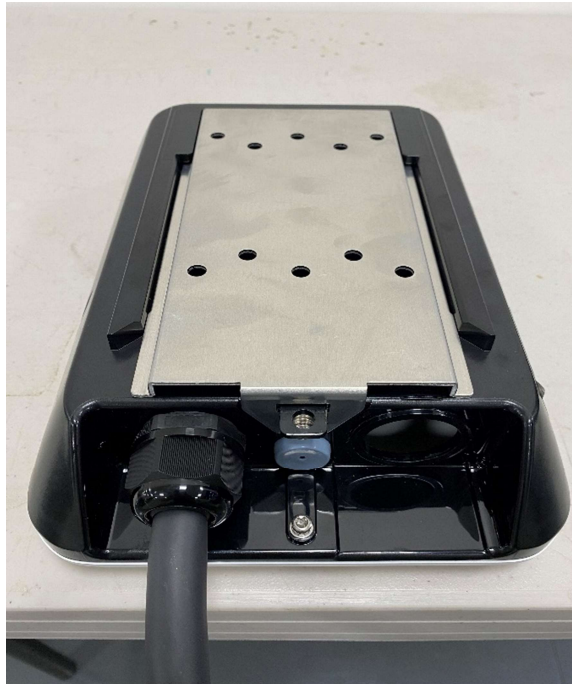
Figure 1-9 Release the screw
