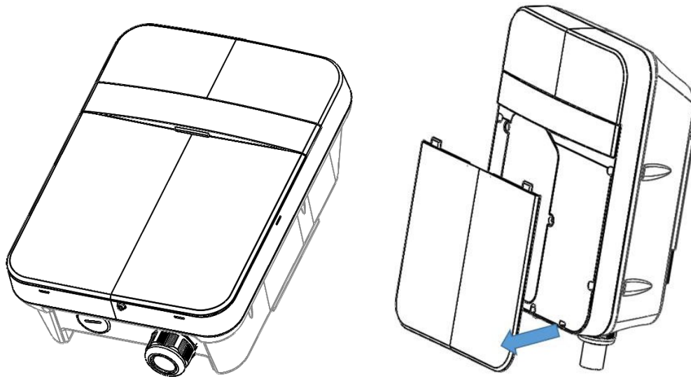
Figure 3-2 Use flat tip screw driver to push snap then open front cover.
