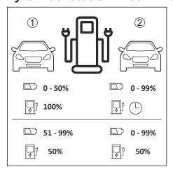
When the EVSE is configured for First In First Served (FIFO) power allocation, it can serve two EVs at a time with DC fast charging.
