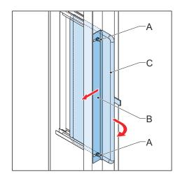
5. Carefully pull and remove the outlet filter (C).
