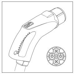
The manufacturer can deliver the EVSE with CHAdeMO connectors on the EV charge cables.
