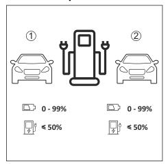
When the EVSE is configured for concurrent power allocation, it can serve two EVs at a time with DC fast charging.
