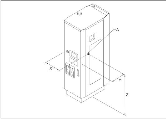
A Center of gravityX Location of A in EVSE width
