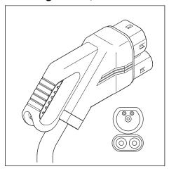
The manufacturer can deliver the EVSE with CCS 2 connectors on the EV charge cables.
