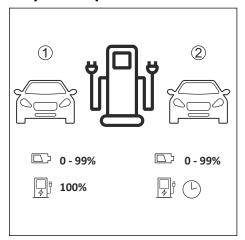
When the EVSE is configured for sequential power allocation, it can serve one EV at a time with DC fast charging.
