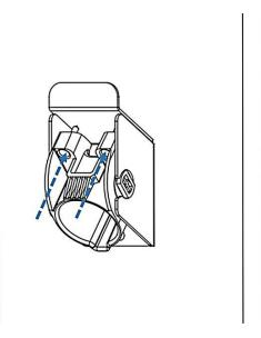
Figure 3-20 Tighten screws
