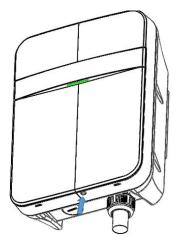
Figure 3-1 Loosen 1 pc M4 screw.
