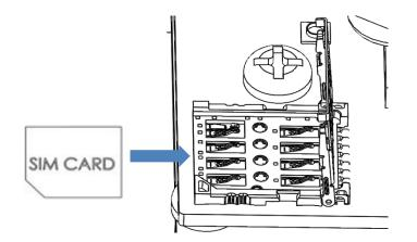
Figure 3-7 input the SIM Card
