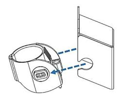
Figure 3-16 Separate the holster
