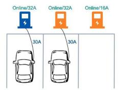
With three connected vehicles, the charging currents are further reduced to 24A for 32A charging stations and the charging current is 12A for 16A charging station.
