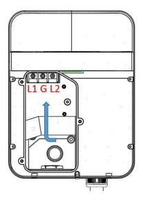
Figure 3-15 Input wiring position.
