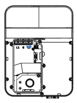
Figure 3-4 Position of SIM card socket
