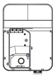
Figure 3-11 Tighten M6 screw
