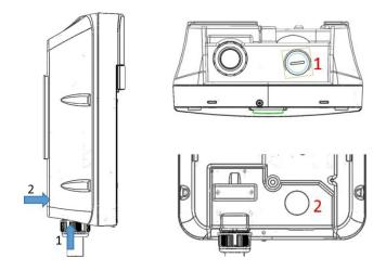
Figure 3-14 Cable input position
