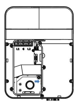
Figure 4-1 Location of Ethernet RJ-45 port
