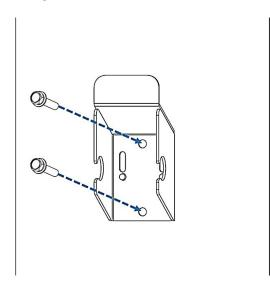
Figure 3-17 Secure the hook
