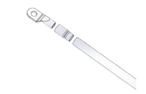
Figure 3-13 Copper terminal, heat shrink tube and copper wire.
