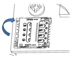
Figure 3-6 open the socket cover
