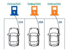
When the first vehicle left, the second vehicle would receive 32A, and the third vehicle would receive 28A.
