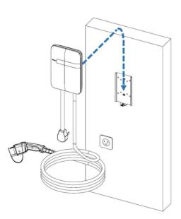
Figure 3-11 Charge point and mounting bracket
