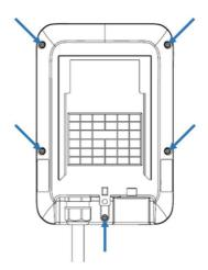
Figure 3-1 Five screws in the Base Cover position
