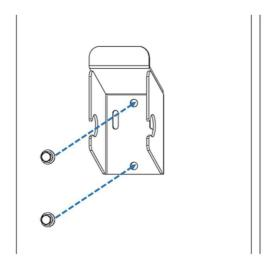
Figure 3-20 Secure the hook
