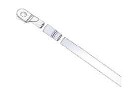
Figure 3-16 Copper terminal, heat shrink tube and copper wire.
