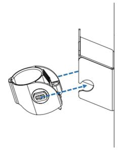
Figure 3-21 Secure the holster
