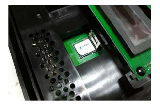
Figure 3-6 Insert the SIM card
