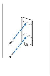
Figure 3-9 Fixing mounting bracket
