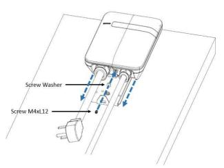
Figure 3-12 Screw locking position
