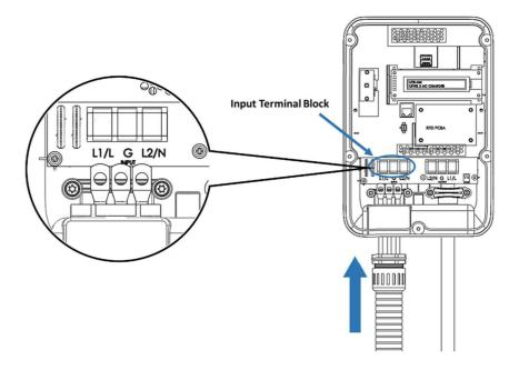
Figure 3-18 Input wiring
