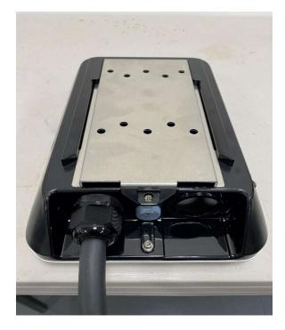
Figure 1-9 Release the screw
