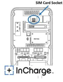
Figure 3-2 Position of SIM card socket
