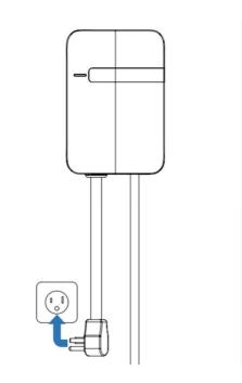
Figure 3-13 Plug in the power cord
