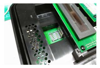
Figure 3-4 Open SIM card socket
