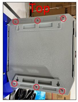
Next, place the charger is on its side and attach the two backets, that were supplied with the ICE-30 charger, on to the back side using the six smaller screws provided in the parts bag. Please note that the large holes on the bracket should be on the south side, while the tracks face north.
