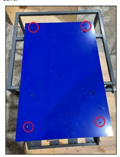
• Once the back plate has been lined up, Screw in the four 1-4'-20 x 34' the holes that
