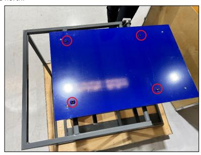
Next, take the four 3/8-16 x ¾" screws, and install them into remaining four holes on the backplate. Please note that the screws should only be tightened enough to allow the bracket to slide in place, and not tightened all the way.
