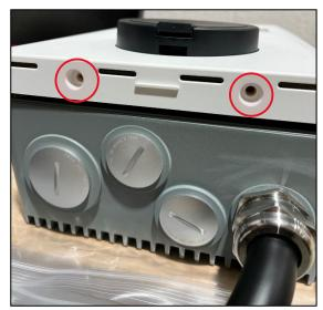
Once the device has been removed from the box, start by removing the two T24 security screws from the bottom of the white cover.
