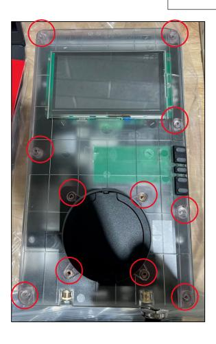
After the white cover has been removed, remove the clear cover by unscrewing the 11
