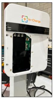
• After placing the charger back onto the bracket, place the screw back into place and assure that the charger is secure to the pedestal.
