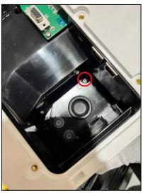
Once this screw has been removed, the bracket will slide right off the back end.
