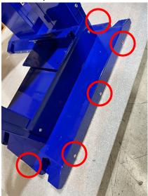
■ Insert and screw in 5 of provided screws per side to secure U covers in place.
