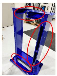
• After the AC Input wires have been installed through the bottom and right side of the pedestal. Place the remaining covers on the pedestal using 7 of the provided screws.
