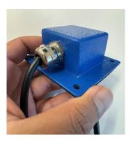
Run the supplied cable harness through the gland nut and out the bottom of the new top cover.
