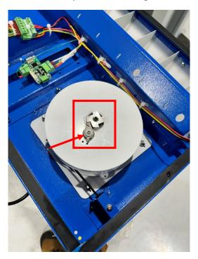
To adjust the cable retractor for different cables, use a 6mm Hex wrench and use your thumb to release the buckle on the left side of the adjustment nut (Please use caution when adjusting and wear appropriate PPE. Once the tension starts building up, the risk of an accident increases). Adjust the tension by turning clockwise to increase tension and counterclockwise for decreasing tension. Each turn will be 90 degrees to adjust the setting by one (One rotation).
