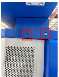
Carefully lay the light bar in line with the holes at the top rim of the charger and screw the four provided Phillips head screws into place (Two on each side) (DO NOT SECURE WITH THE PLASTIC SCREWS THAT COME ON THE EVSE TO SECURE THE LIGHT BAR). Please note that the wires should not be pinched by the bracket (the wire harness should be tucked within the bracket).
