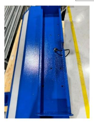
• Flip the light bar upside down and insert the 8 bolts that secure the light bar to the bracket.
