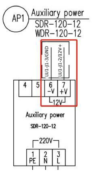
Connect the Red (LU-J1-2/12V+) and Green/Yellow (LU1-J1-3/GND) wires as shown in the diagram above. The Red wire lands in the 7<sup>th</sup> port (V+) and the Green/Yellow wire lands in the 6<sup>th</sup> port (V-).
