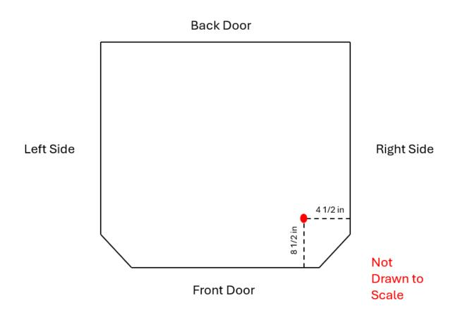
Above is an image showing where to mark the hole of the pass through on the ICE 60/120/180 (Top View).
