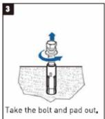
■ Drilling instructions: Drill out 4 holes 60mm-80mm (2.36in – 3.15in) and clear out debris. Knock the bolt with anchor into place with a hammer. Then, take the bolt and pad out.
