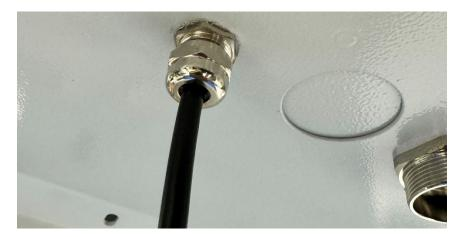
• Run the light bar wire harness into the bottom of the ICE-30.
