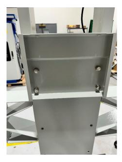
Take the supplied bracket and mount it in the position as shown above using the four M10\*30 bolts.
