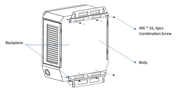
Figure 6: ICE-30 Bracket bolt pattern
