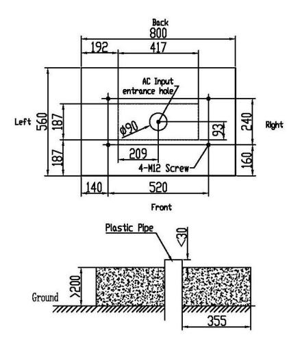
Figure 9: Concrete foundation view
