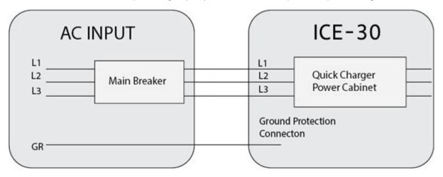
Figure 11: AC Input Wiring
