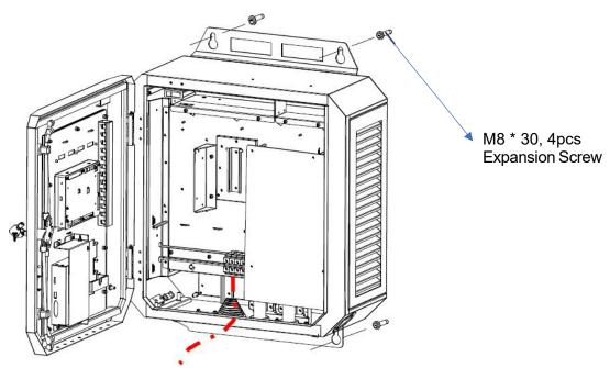
Figure 7: Grid input wiring
