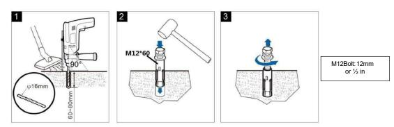
Figure 8: Anchor Installation
