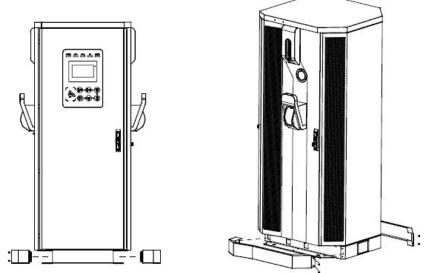
Align the installation hole of the cabinet base and fix the cabinet to the concrete foundation with expansion bolts.
