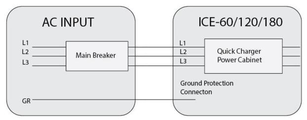
Figure 14: AC Input Wiring
