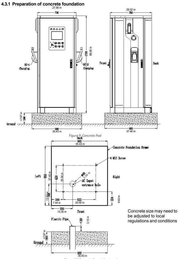
Figure 10: Concrete foundation top view
