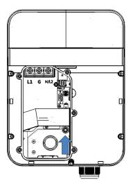
Figure 3-11 Tighten M6 Screw
