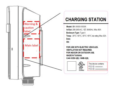
Figure 4-1 Serial Number on the Main Label
