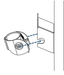
Figure 3-18 Secure the Holster
