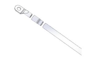
Figure 3-13 Copper Terminal, Heat Shrink Tube and Copper Wire
