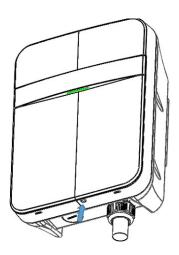
Figure 3-1 Loosen 1 pc M4 Screw
