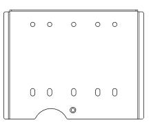
Figure 3-9 Screw Holes of Mounting Bracket
