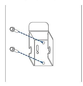
Figure 3-17 Secure the hook
