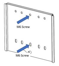
Figure 3-8 Fasten Mounting Bracket
