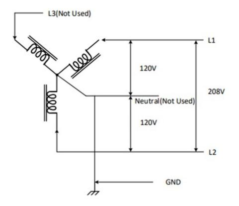
Figure 3-23 208V 3-Phase WYE-Connected
