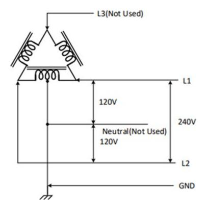
Figure 3-24 240V 3-Phase Delta-Connected
