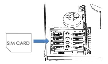
Figure 3-7 Input the SIM Card
