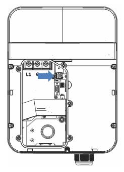
Figure 3-4 Position of SIM Card Socket
