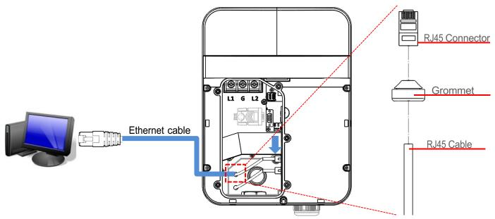
Figure 4-2 Connect the Laptop with Charge Point Directly with an Ethernet Cable
