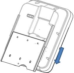
Figure 1-6 Remove the Mounting Bracket
