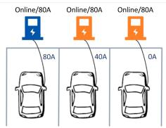
When the first vehicle left, the second vehicle would receive 80A, and the third vehicle would receive 40A.
