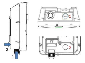
Figure 3-14 Cable Input Position
