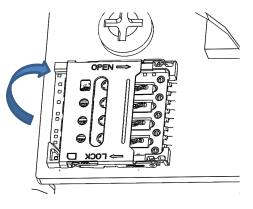
Figure 3-6 Open the Socket Cover
