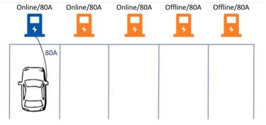
The second vehicle would also receive 80A, due to the total current doesn't exceed the max amperage grid connection. (Reserve 20A for offline charging stations)
