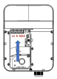
Figure 3-15 Input Wiring Position
