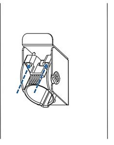
Figure 3-20 Tighten Screws
