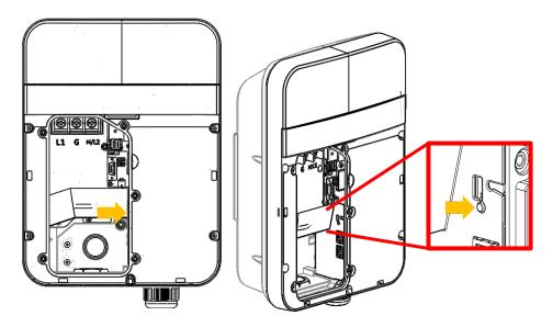
Figure 4-20 The Hardware Reset Button
